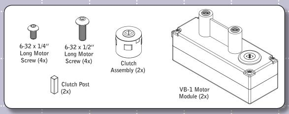
The VB-1 Motor comes with an optional Clutch Assembly. This clutch mounts on top of the VB-1 Motor, protecting the Motor from any sudden "shock loads". To install the clutch, insert a clutch post into the square hole motoroutput, and then insert the clutch on top of this clutch post.
