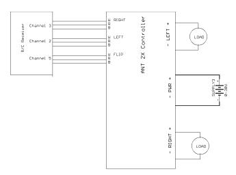
Typical wiring diagrams are shown above. Note that channel assignments will vary depending upon the radio gear used.
