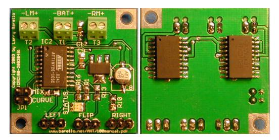
The Ant 100 R/C Robot Controller offers unparalleled functionality and reliability for your creation with dual motor drive, selectable single stick control, Adjustable control curve and a FLIP input that reverses and swaps the motor drive output for robots that are invertible.
