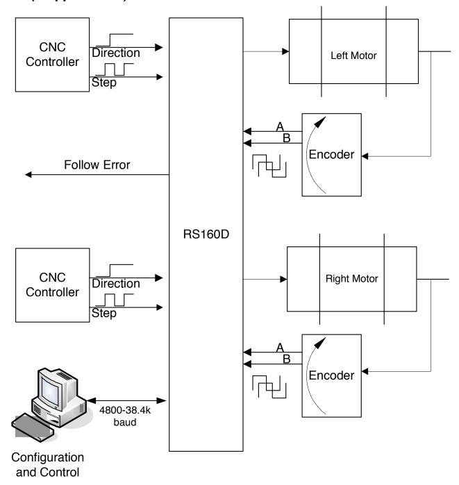
CNC Step control advances the position set point +/- one count for each 0 to 5v step input. 0v direction = reverse, 5v direction = forward. Three channels of CNC control are available on the RS160D with the addition of a third OSMC motor driver board.
