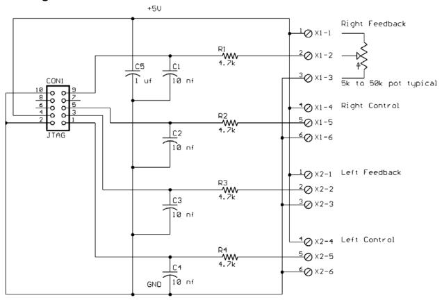
Analog signals are shared with the JTAG programming interface (non-latched 10 pin connector behind the AUX OSMC connector). The above interface can be used for mechanical (potentiometer) connections.
