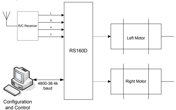
Factory default configuration supports traditional differential drive remote control robot operation (Combat robots, for example). The default configuration enables channel mixing so the LEFT input controls overall speed and the RIGHT input controls steering.
