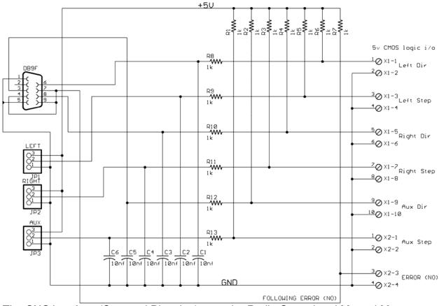
The CNC interface (Step and Direction) uses the Radio Control and Manual Move interface to supply the input signaling connections. The Radio Control connectors provide the high speed step input and the manual move interface provides the direction input and following error outputs for each channel.
