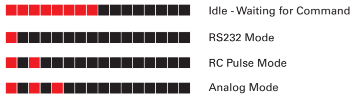
FIGURE 12. Normal Operation Flashing Patterns
