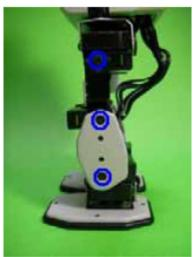
5. Set the origins of the thighs' pitch, the knee pitch and the ankle pitch for both legs while keeping the screws of each joint (indicated in blue circles in the left picture) aligned straight.
