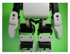
2. Set the origins of both arms' roll and the roll of the elbow while keeping the arms and the forearms aligned straight.
