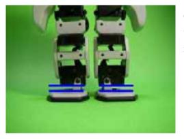
6. Set the origin of both ankles' roll while keeping the servo and the leg parallel as shown in blue lines in the left picture.
