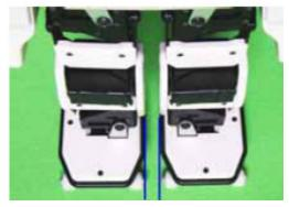
3. Set the origins of both thighs' yaw while keeping both feet parallel to each other as shown in blue lines in the left picture.
