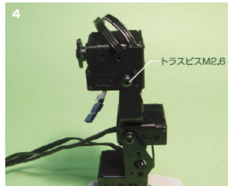
4 Insert one Round top M2.6 screw
