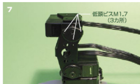
Lock down the servo motor with 3 M1.7 screws as shown
