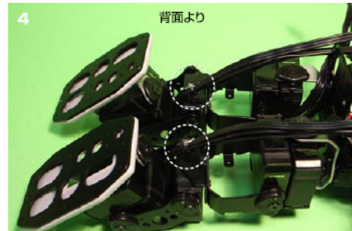
Band the Knee Servo Unit cable to the banded Ankle Servo Unit cables at the base of the Knee Servo Unit cable as shown (both legs). ie [R16 to R17/18] and [L04 to L05/06].
