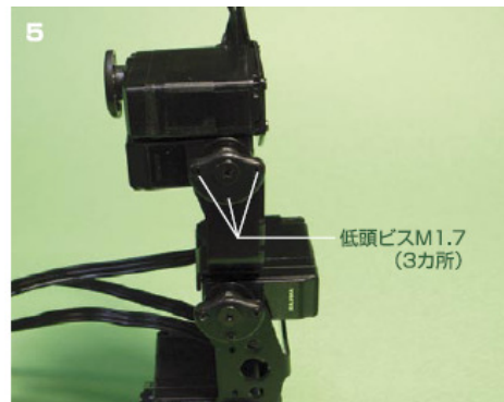
Attach the Servo Joint and secure using M1.7 Flat top screw
