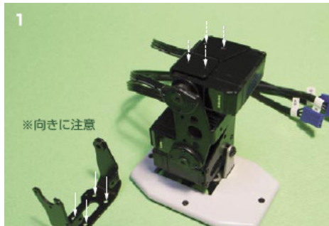
Attach R Thigh Frame to the R Knee Servo Unit and secure using M2×2.5 Flat top screw (x4)
