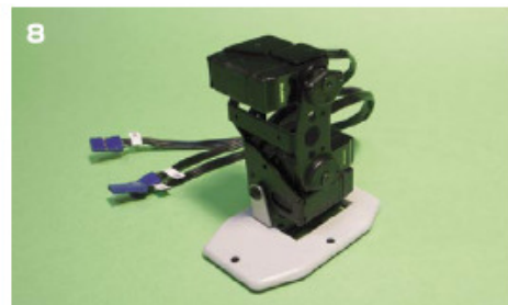
Lock down the servo motor with 3 M1.7 screws as shown
