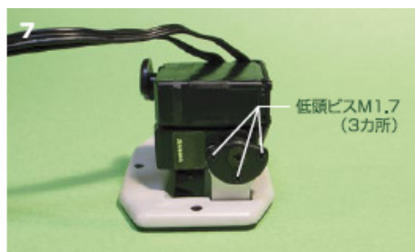
Lock down the servo with 3 M1.7 Flat head screws
