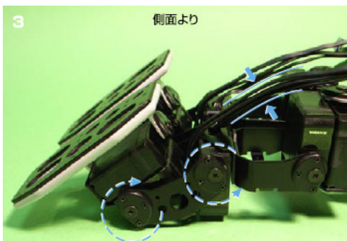
Position the ankle joints as shown (soles up). Group the cables together behind the knee (do the same on both the left and right leg).
