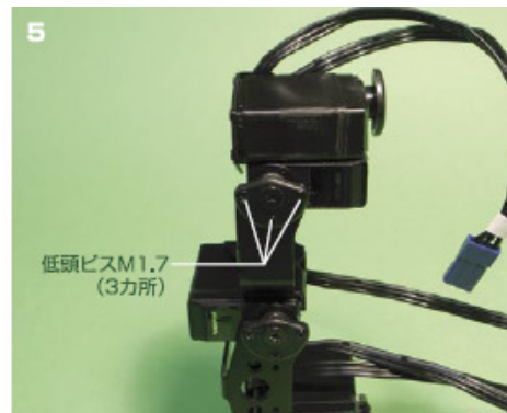
5 Lock down the servos with 3 M1.7
