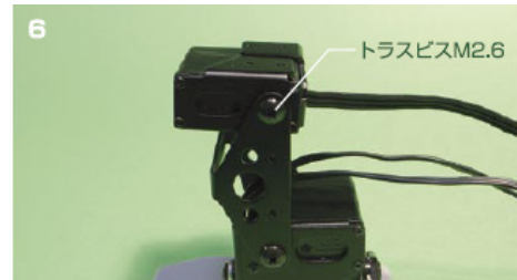
Secure using M2.6 Round top screw
