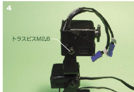
Secure using M2.6 Round top screw
