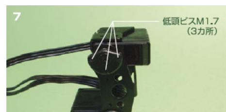
Attach the Servo Joint and secure using M1.7 Flat top screw
