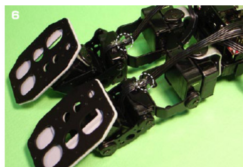
Pass the banded group of cables (from step 4.above) over the Knee Frame and cable tie to secure using the loose Vinyl Cord (on the upper side of the Knee Frame) as shown (both legs).
