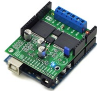
Pololu dual VNH5019 motor driver shield, assembled and connected to an Arduino Uno.
