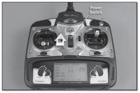
❑ Your Novus helicopter uses a 2.4GHz system that requires linking the transmitter to the receiver when the unit is powered up. With the transmitter turned **off**, connect the flight battery to the helicopter. Then place the model on a flat surface and turn the transmitter on. You will notice that the trim tab indicators are moving. This is an indication of the linking process. Allow the helicopter to remain still and do not move the transmitter sticks during the linking process.
