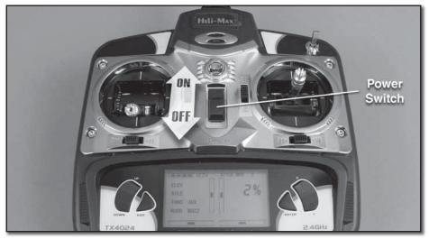
Turn on the transmitter and verify that the LCD initializes. Turn the transmitter off for now. If the LCD did not initialize, remove the battery box from the transmitter and verify that the batteries were installed correctly
