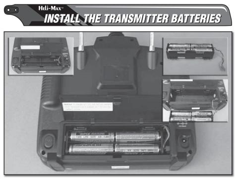
□ Open the battery cover on the back of the transmitter, remove the battery box and install eight AA batteries into the battery box. Double check the polarity of each battery before placing the battery box back into the transmitter and replacing the battery cover.
