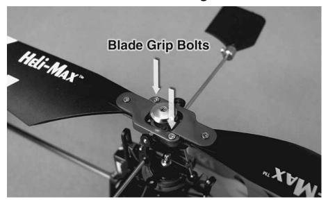
It has been found that the two bolts shown above may come loose during normal use. To prevent this from occurring the following steps must be performed. Remove one bolt and apply thread locker to the screw (GPMR6060 Great Planes Pro Threadlocker is recommended). Reinstall and tighten the screw. Repeat the steps for the other screw.
