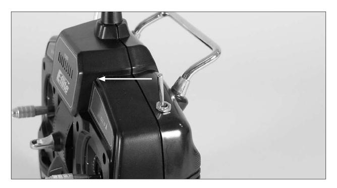
**Note**: When in stunt mode, even with the throttle stick all the way down, the blades and motors will continue to spin. You must use the normal flight mode to safely turn off the motors. For safety, the 3-in-1 unit will not arm if the flight battery is plugged in and the flight mode switch is in the stunt position.
