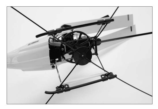
• Install one plastic ball on the exposed end of each rod. Then, slide one tubing keeper over the end of each rod to prevent the ball from sliding off. Adjust the position of the tubing keepers that were factory-installed on each rod until they are just touching each plastic ball. The tubing keepers should then be positioned so that the ball can spin freely on the rod, without too much movement side-to-side between the keepers.
