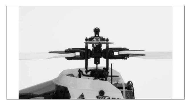
• Once you have positioned the flybar paddles correctly following the steps above, be certain they are firmly secured using the included screws, washers and hex nuts.
