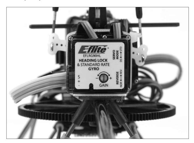
Once you have made initial adjustments of the gyro gain setting, you will be ready to conduct the first
