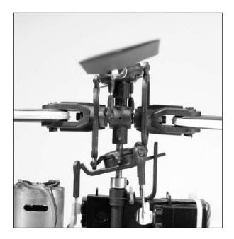
With the stick pulled back, the swashplate will tilt toward the rear.
