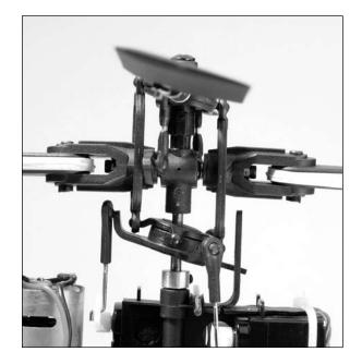
While viewing the helicopter from the rear (tail boom toward you), move the right-hand stick left and right to check aileron roll control. When the stick is pushed to the left, the swashplate should also tilt left.
