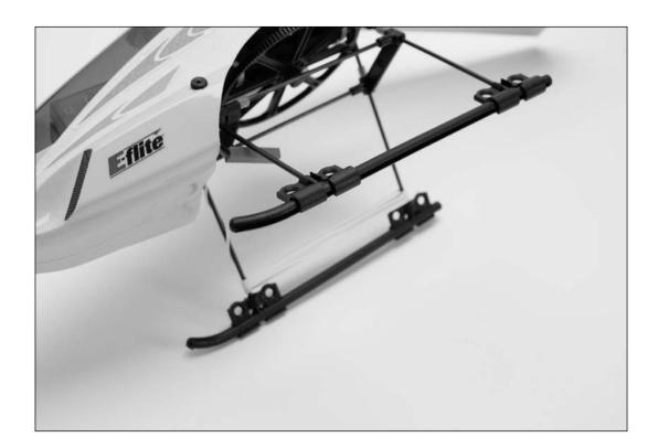
• After installing all four attachments, locate the four training gear rods and rod mounting base. Note that the rod mounting base has four channels into which the training gear rods will mount. The "open" side of these channels will face upward toward the bottom of the helicopter when properly installed.
