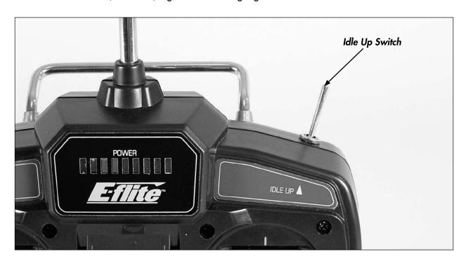
With the switch toggled toward the rear of the transmitter, the Blade CP+ will be flying in "normal mode." In this flight mode, the throttle curve is linear from 0% to 100%, with a pitch range of 0 degrees to +10 degrees. (See Page 40 for additional data and graphics relating to the throttle and pitch curves preset for your Blade CP+.) This is the preferred flight mode for general hovering and gentle forward flight.
